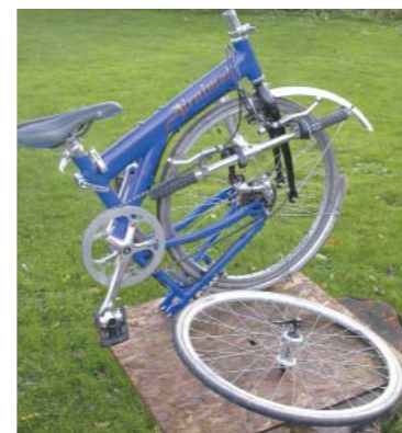
BELOW: The folded package is by no means small, but it's an easy process. The front mudguard might be better removed.
